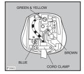
The wire coloured green and yellow must be connected to the terminal marked with the letter «E» or by the earth symbol  $\frac{1}{2}$  or coloured green and yellow.
